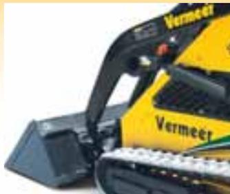
*Curved loader arms lift up and away from the machine, providing better height and reach for loading and unloading. This also provides the clearance necessary to avoid damaging the front of the machine when using large-diameter augers and allows an operator to dump a bucket into the center of a one-ton truck.*
