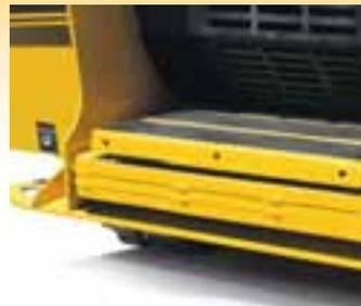
*The ride-on unit comes with a spring-cushioned platform, keeping the operator out of mud and debris. At 14.5" (36.8 cm), it is high enough to enhance visibility while providing clearance for backing over curbs.*
